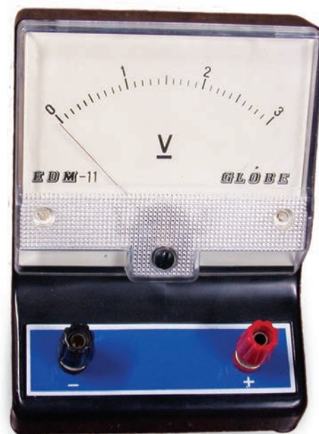
Figure 1.8 Voltmeter with zero error
