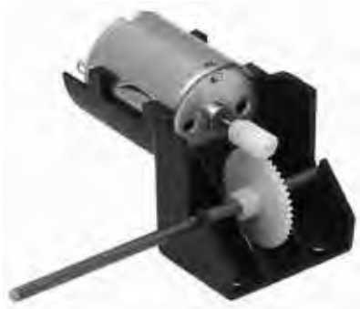
A gearbox can be used to convert the high speed of the motor to a slower speed.
